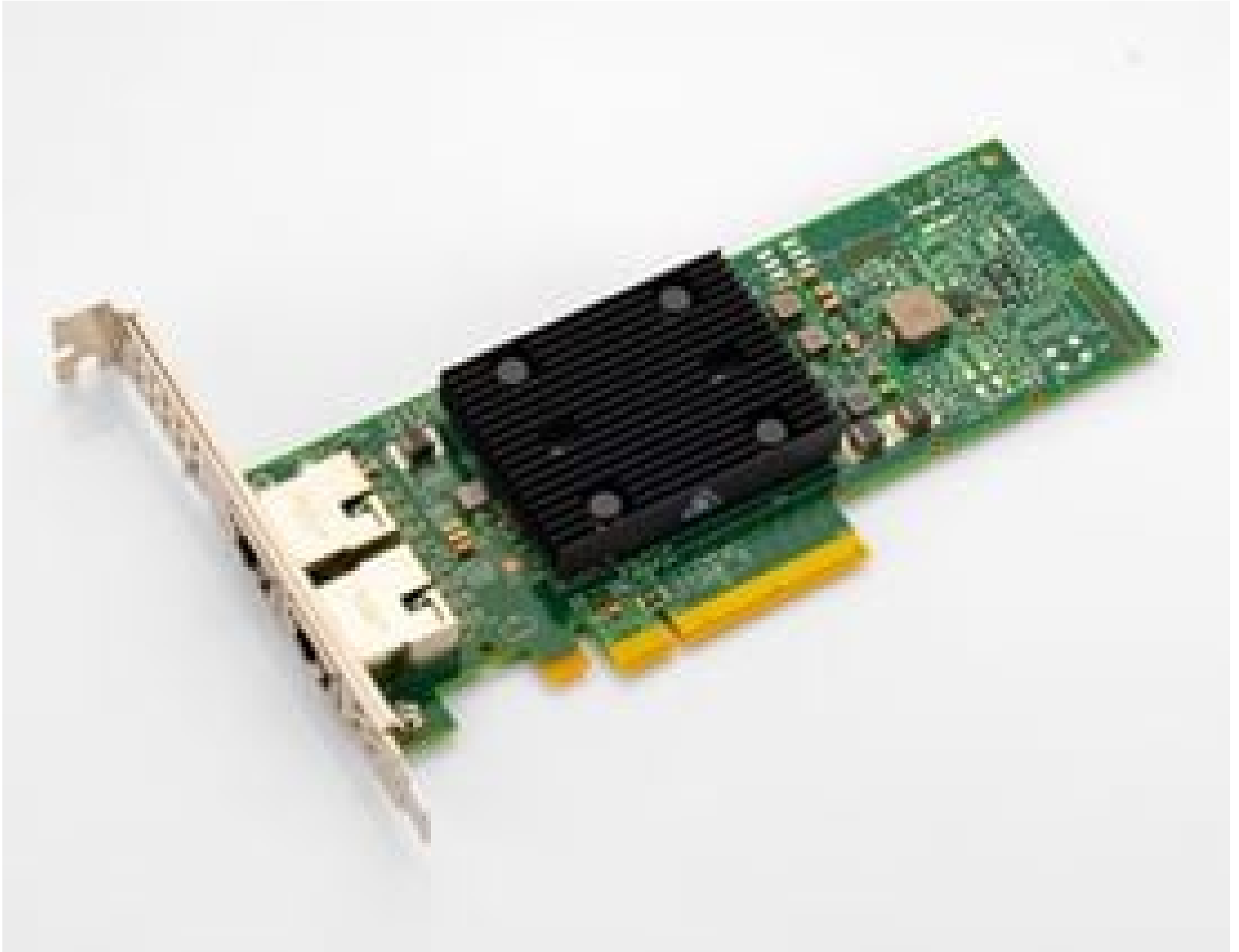
Broadcom Dual Port 10G Ethernet Card
