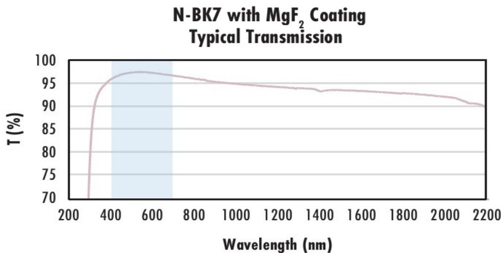
Typical transmission of a 3mm thick N-BK7 window with MgF<sub>2</sub> (400-700nm) coating at 0° AOI.
