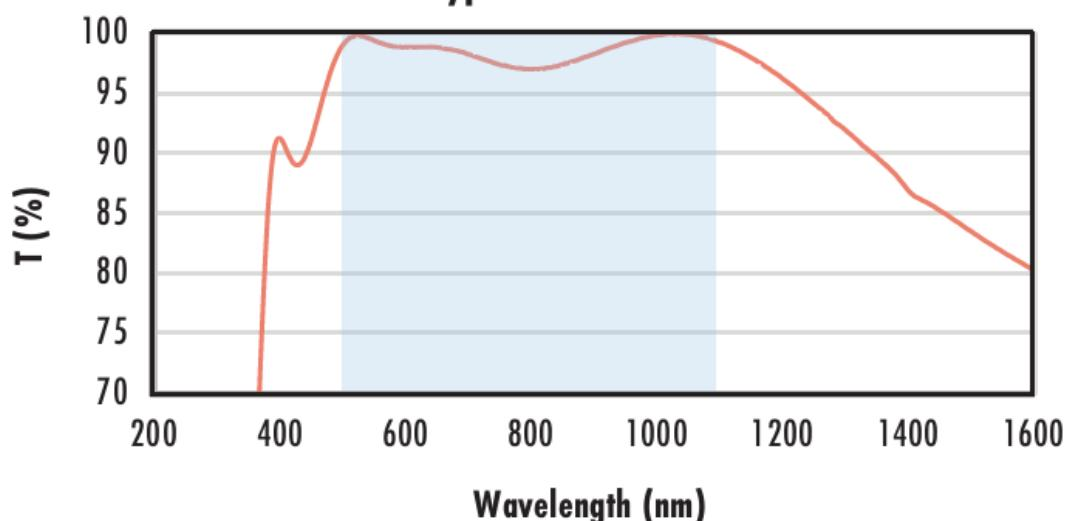
Typical transmission of a 3mm thick N-BK7 window with YAG-BBAR (500-1100nm) coating at 0° AOI.
