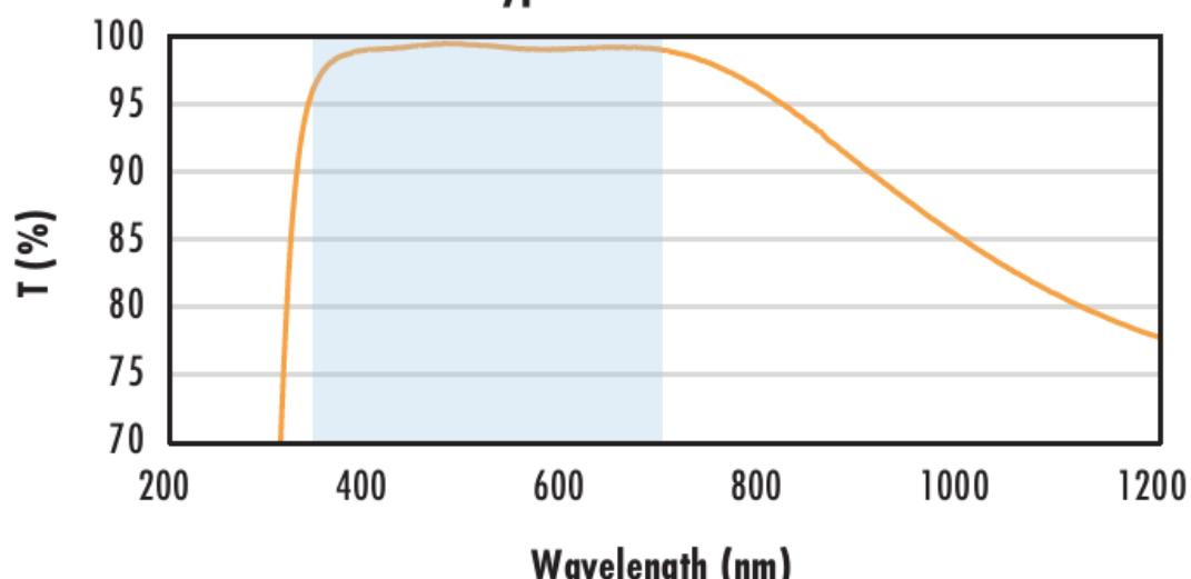
Typical transmission of a 3mm thick N-BK7 window with VIS-EXT (350-700nm) coating at 0° AOI.
