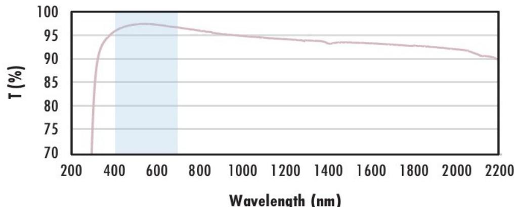
Typical transmission of a 3mm thick N-BK7 window with MgF2 (400-700nm) coating at 0° AOI.
