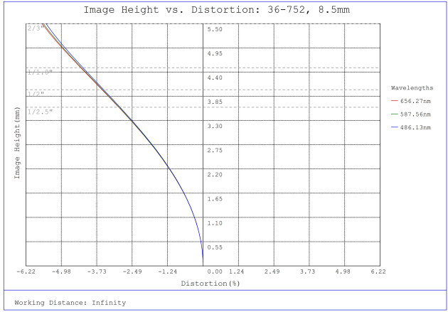
#36-752, 8.5mm f/8, 75mm-∞ Primary WD, HRi Series Fixed Focal Length Lens, Distortion Plot
