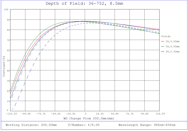
#36-752, 8.5mm f/8, 75mm-∞ Primary WD, HRi Series Fixed Focal Length Lens, Depth of Field Plot, 200mm Working Distance, f8
