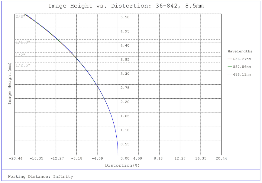
#36-842, 8.5mm, f/5.6 Cr Series Fixed Focal Length Lens, Distortion Plot
