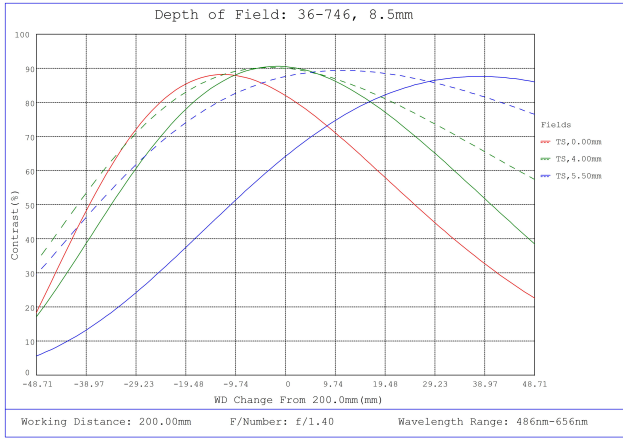
#36-746, 8.5mm f/1.4, 75mm-∞ Primary WD, HRi Series Fixed Focal Length Lens, Depth of Field Plot, 200mm Working Distance, f1.4
