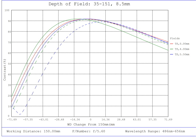
#35-151, 8.5mm, f/5.6, 75mm-∞ Primary WD, HRr Series Fixed Focal Length Lens, Depth of Field Plot, 150mm Working Distance, f5.6
