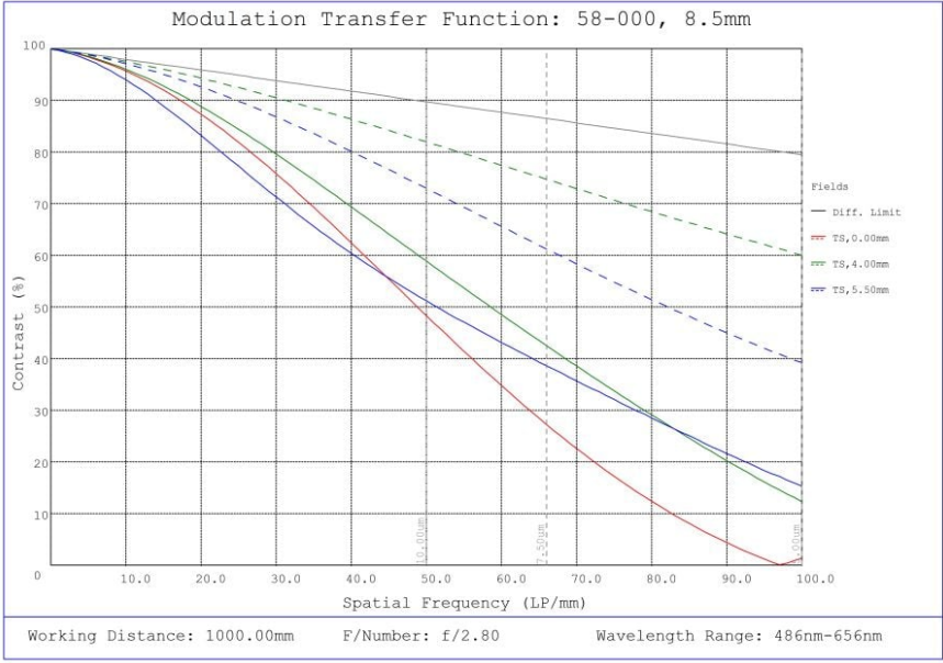
#58-000, 8.5mm C Series Fixed Focal Length Lens, Modulated Transfer Function (MTF) Plot, 1000mm Working Distance, f2.8
