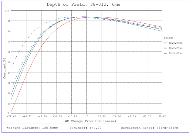
#38-012, 6mm FL f/4, Blue Series M12 Lens, Depth of Field Plot, 150mm Working Distance, f4
