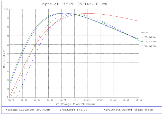
#35-142, 6mm, f/4 Cr Series Fixed Focal Length Lens, Depth of Field Plot, 200mm Working Distance, f4
