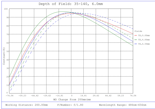
#35-140, 6mm, f/1.8 Cr Series Fixed Focal Length Lens, Depth of Field Plot, 200mm Working Distance, f1.8
