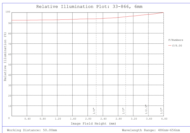
#33-866, 6mm, f/8 UCi Series Fixed Focal Length Lens, Relative Illumination Plot
