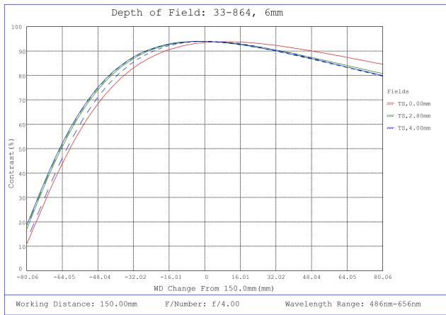
#33-864, 6mm, f/4 UCi Series Fixed Focal Length Lens, Depth of Field Plot, 150mm Working Distance, f4
