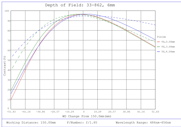
#33-862, 6mm, f/1.85 UCi Series Fixed Focal Length Lens, Depth of Field Plot, 150mm Working Distance, f1.8
