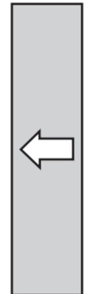
All mounted TECHSPEC® Optical Filters have an arrow on the side of the mount that points to the filter-coated surface for quick reference. Filter oriented such that arrow points to filter coated surface S1.
