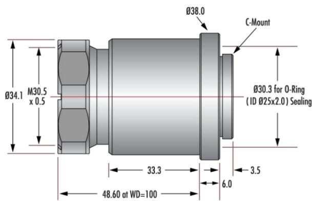
16mm Cw Series Fixed Focal Length Lens
