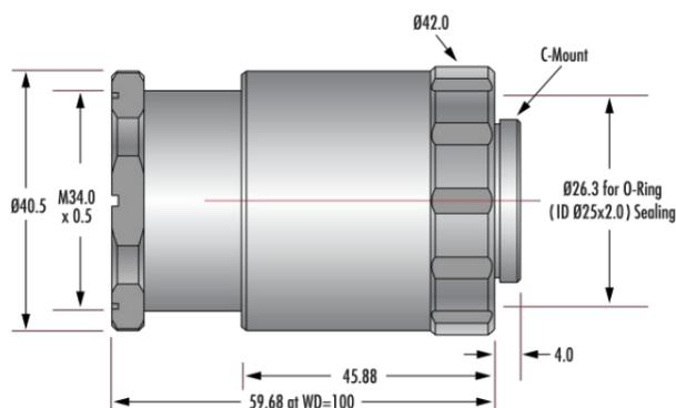
35mm Cw Series Fixed Focal Length Lens
