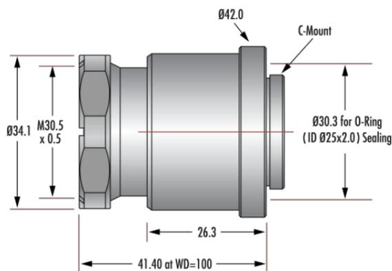
25mm Cw Series Fixed Focal Length Lens
