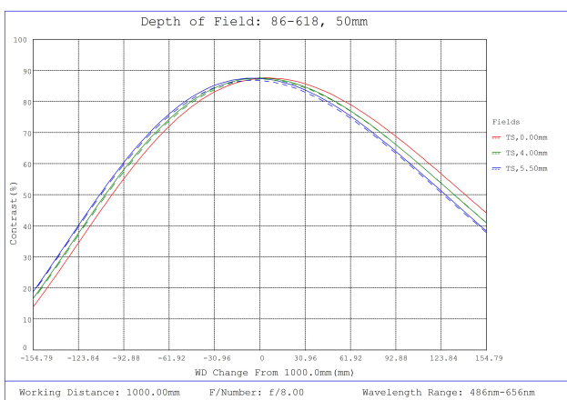
#86-618, 50mm, f/8.0 Ci Series Fixed Focal Length Lens, Depth of Field Plot, 1000mm Working Distance, f8
