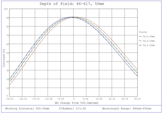
#86-617, 50mm, f/5.6 Ci Series Fixed Focal Length Lens, Depth of Field Plot, 500mm Working Distance, f5.6
