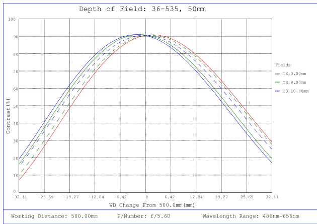
#36-535, 50mm f/5.6, HPr Series Fixed Focal Length Lens, Depth of Field Plot, 500mm Working Distance, f5.6
