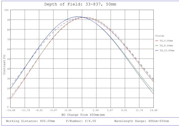
#33-837, 50mm f/4.0, HPI Series Fixed Focal Length Lens, Depth of Field Plot, 400mm Working Distance, f4
