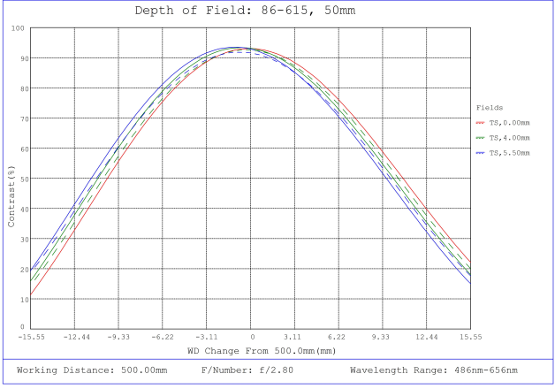
#86-615, 50mm, f/2.8 Ci Series Fixed Focal Length Lens, Depth of Field Plot, 500mm Working Distance, f2.8
