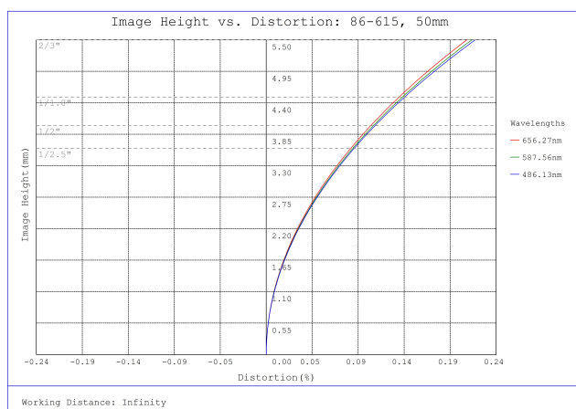
#86-615, 50mm, f/2.8 Ci Series Fixed Focal Length Lens, Distortion Plot
