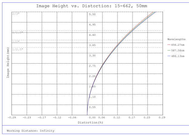
#15-662, 50mm, f/2.0 Sealed Cw Series Fixed Focal Length Lens, Distortion Plot
