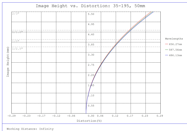
#35-195, 50mm, f/11 Cr Series Fixed Focal Length Lens, Distortion Plot
