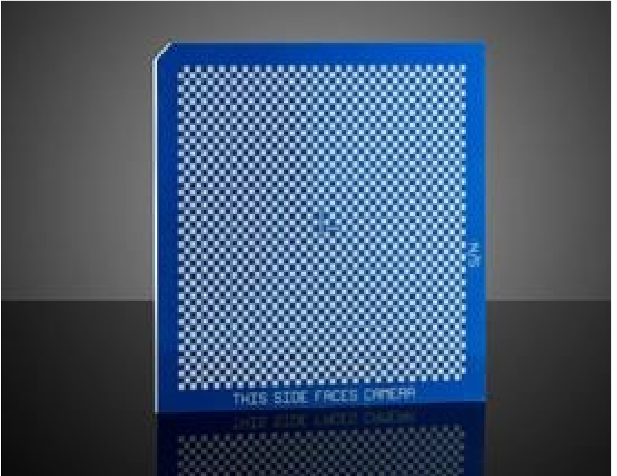
Opal Checkerboard Calibration Target
