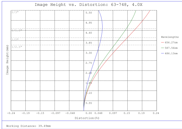
#63-748, 4X, 40mm WD CompactTL™ Telecentric Lens, Distortion Plot
