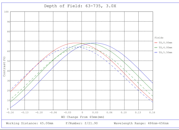
#63-735, 3X, 65mm WD CompactTL™ Telecentric Lens, Depth of Field Plot, 65mm Working Distance, f21.9
