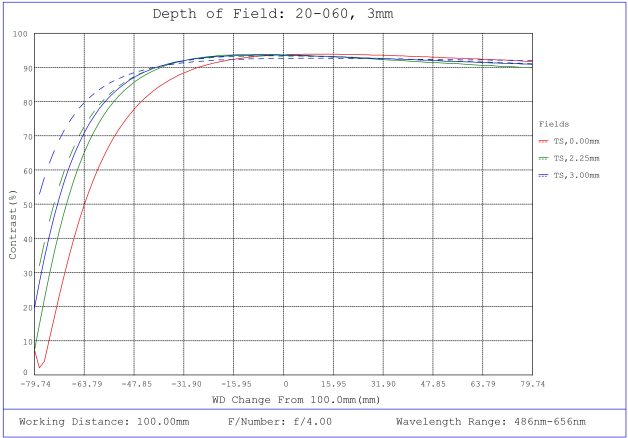
#20-060, 3mm FL f/4.0 IR-Cut Rugged Blue Series M12 Lens, Depth of Field Plot, 100mm Working Distance, f4
