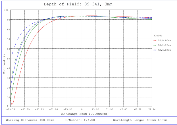
#89-341, 3mm FL f/4.0, Blue Series M12 Lens, Depth of Field Plot, 100mm Working Distance, f4
