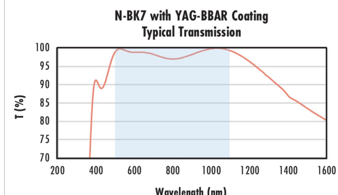
Typical transmission of a 3mm thick N-BK7 window with YAG-BBAR (500-1100nm) coating at 0° AOI.
