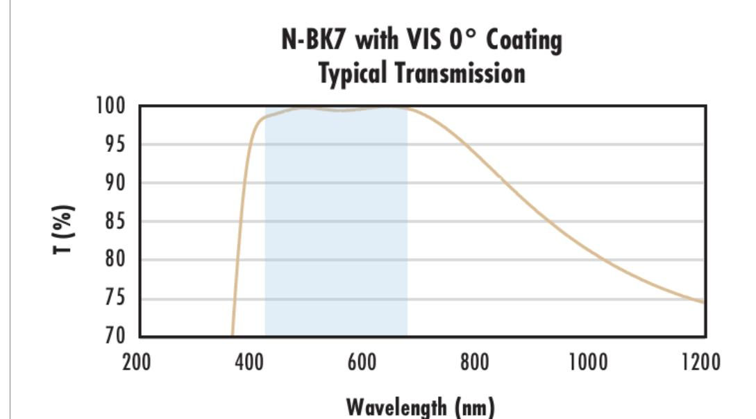
Typical transmission of a 3mm thick N-BK7 window with VIS 0° (425-675nm) coating at 0° AOI.
