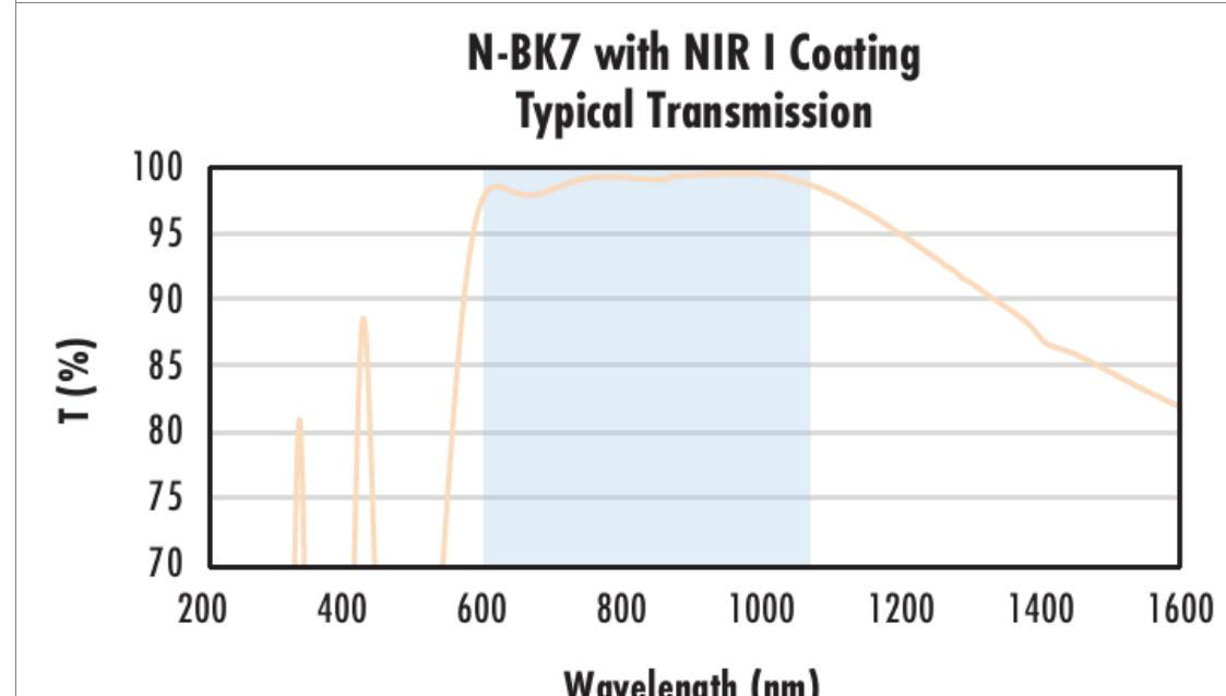
Typical transmission of a 3mm thick N-BK7 window with NIR I (600 - 1050nm) coating at 0° AOI.
