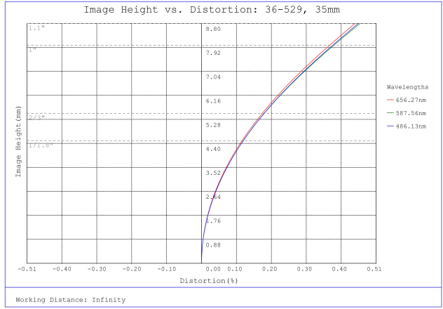
#36-529, 35mm f/5.6, HPr Series Fixed Focal Length Lens, Distortion Plot
