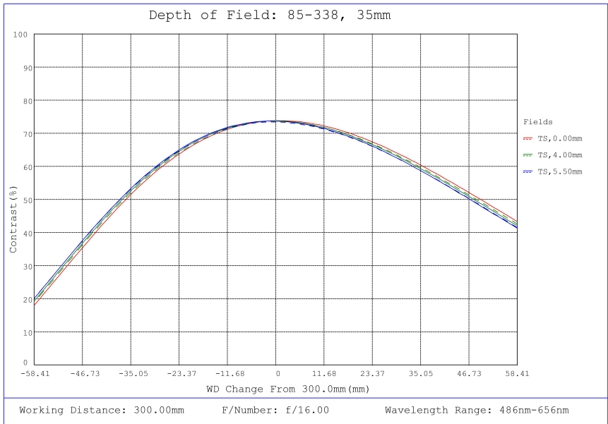
#85-338, 35mm, f/16 Ci Series Fixed Focal Length Lens, Depth of Field Plot, 300mm Working Distance, f16
