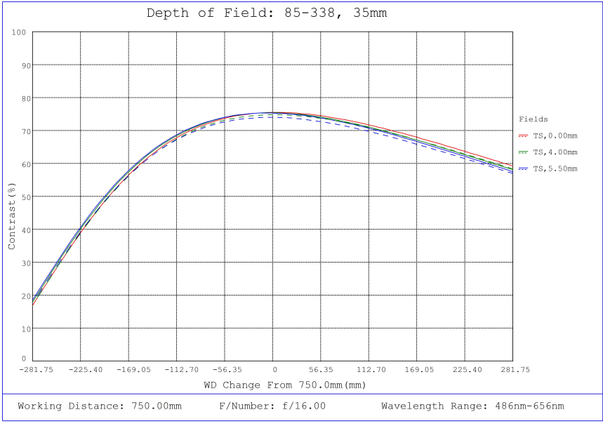
#85-338, 35mm, f/16 Ci Series Fixed Focal Length Lens, Depth of Field Plot, 750mm Working Distance, f16
