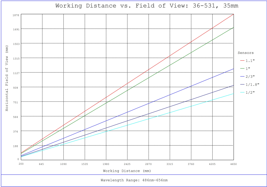
#36-531, 35mm f/11.0, HPr Series Fixed Focal Length Lens, Working Distance versus Field of View Plot
