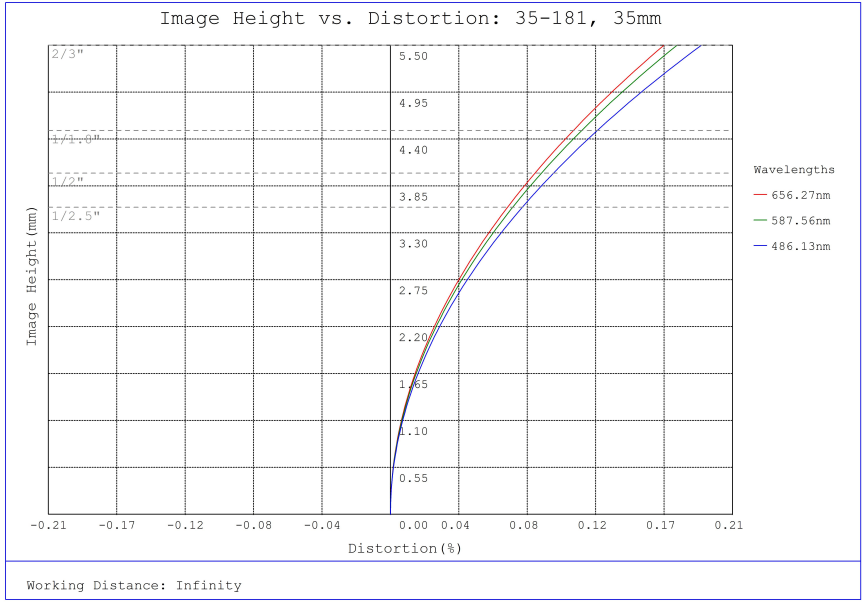
#35-181, 35mm, f/1.65 Cr Series Fixed Focal Length Lens, Distortion Plot
