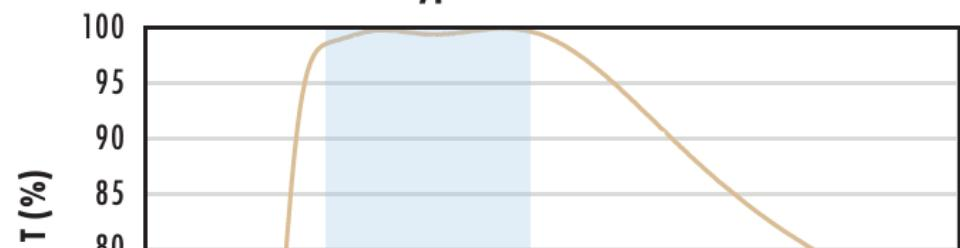
Typical transmission of a 3mm thick N-BK7 window with VIS 0° (425-675nm) coating at 0° AOI.
