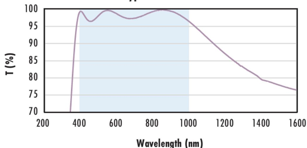
Typical transmission of a 3mm thick N-BK7 window with VIS-NIR (400-1000nm) coating at 0° AOI.
