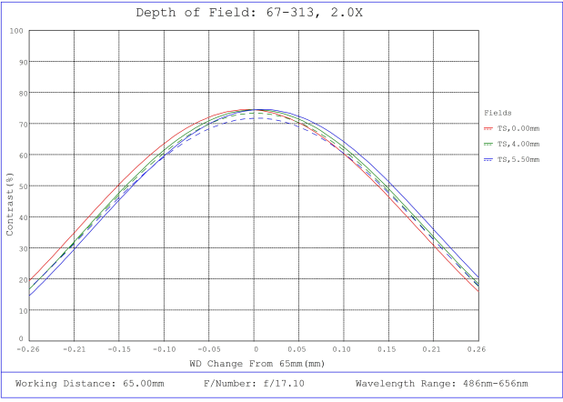
#67-313, 2X, 65mm WD, In-Line CompactTL™ Telecentric Lens, Depth of Field Plot, 65mm Working Distance, f17.1
