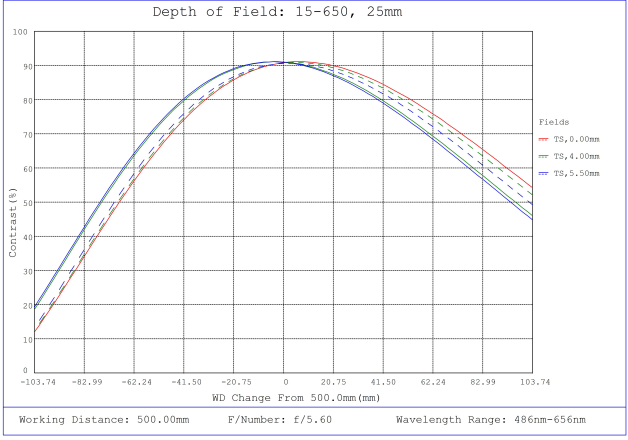
#15-650, 25mm, f/5.6 Cw Series Fixed Focal Length Lens, Depth of Field Plot, 500mm Working Distance, f5.6
