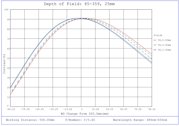
#85-359, 25mm, f/5.6 Ci Series Fixed Focal Length Lens, Depth of Field Plot, 500mm Working Distance, f5.6
