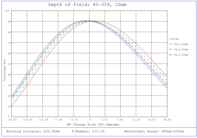
#85-359, 25mm, f/5.6 Ci Series Fixed Focal Length Lens, Depth of Field Plot, 200mm Working Distance, f5.6
