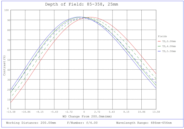
#85-358, 25mm, f/4 Ci Series Fixed Focal Length Lens, Depth of Field Plot, 200mm Working Distance, f4
