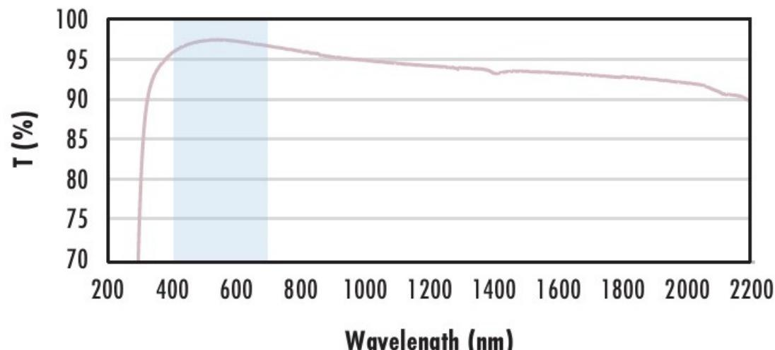
Typical transmission of a 3mm thick N-BK7 window with  $\text{MgF}_2$  (400-700nm) coating at 0° AOI.
