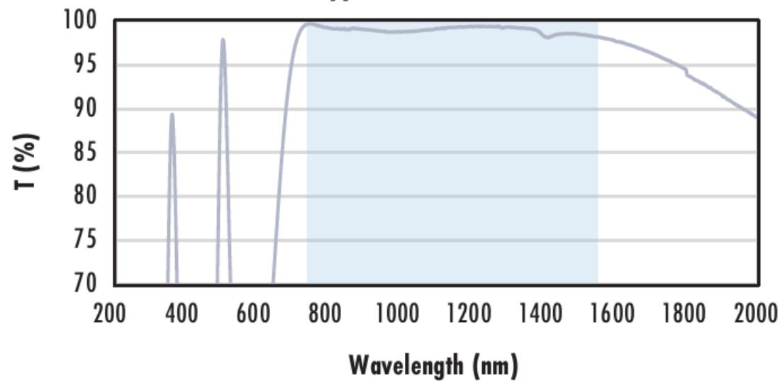
Typical transmission of a 3mm thick N-BK7 window with NIR II (750 - 1550nm) coating at 0° AOI.
