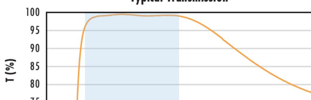
Typical transmission of a 3mm thick N-BK7 window with VIS-EXT (350-700nm) coating at 0° AOI.
