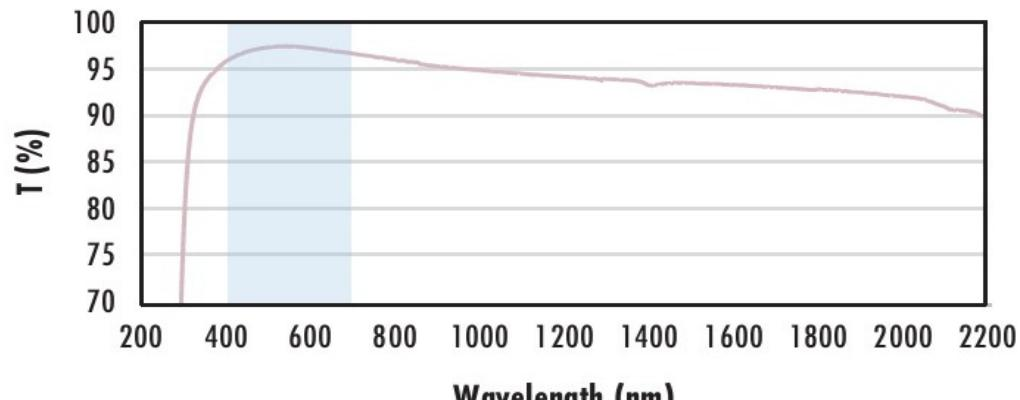
Typical transmission of a 3mm thick N-BK7 window with MgF2 (400-700nm) coating at 0° AOI.
