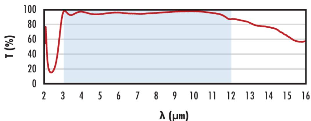
Typical transmission of a 3mm thick Ge window with BBAR (3000-1200nm) coating at 0° AOI.
