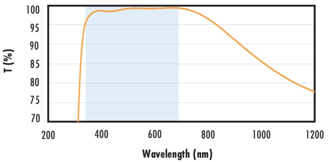
Typical transmission of a 3mm thick fused silica window with VIS-EXT (350-700nm) coating at 0° AOI.
