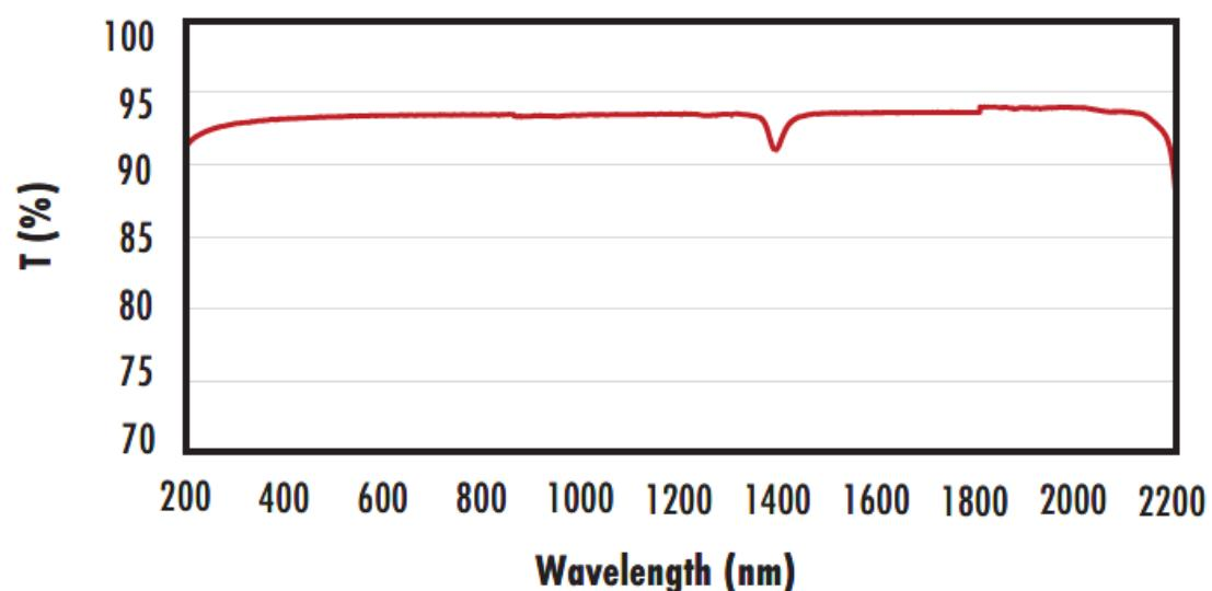
Typical transmission of a 3mm thick, uncoated fused silica window across the UV- NIR spectra.
