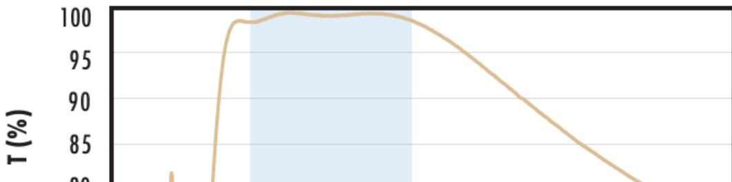
Typical transmission of a 3mm thick fused silica window with VIS 0° (425-675nm) coating at 0° AOI.
