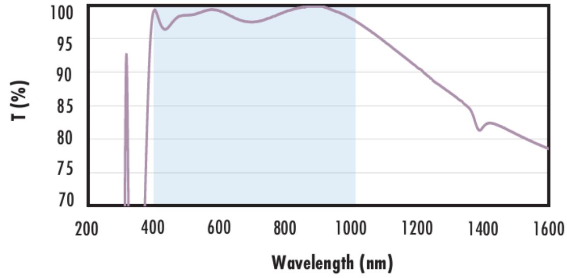
Typical transmission of a 3mm thick fused silica window with VIS-NIR (400-1000nm) coating at 0° AOI.
