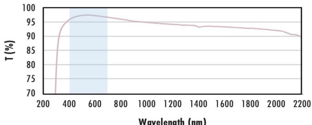
Typical transmission of a 3mm thick N-BK7 window with  $\text{MgF}_2$  (400-700nm) coating at  $0^\circ$  AOI.
