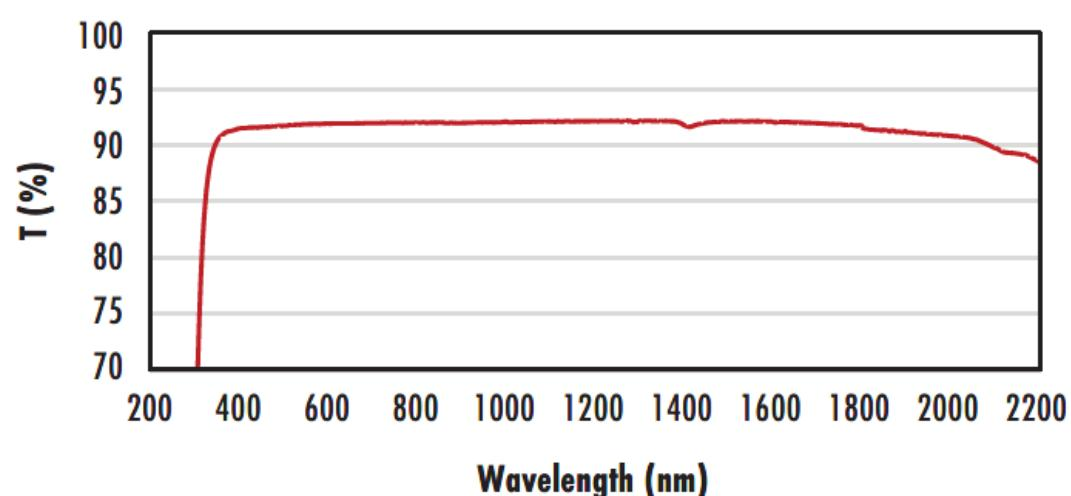
Typical transmission of a 3mm thick, uncoated N-BK7 window across the UV- NIR spectra.
