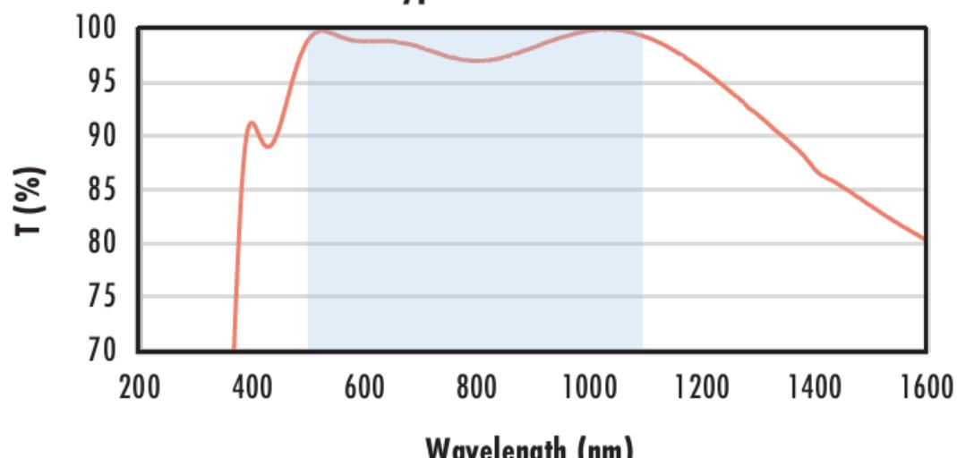
Typical transmission of a 3mm thick N-BK7 window with YAG-BBAR (500-1100nm) coating at 0° AOI.
