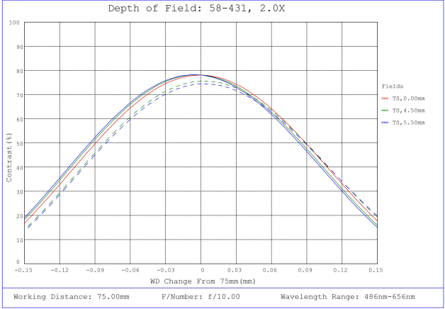
#58-431, 2.0X SilverTL™ Telecentric Lens, Depth of Field Plot, 75mm Working Distance, f10
