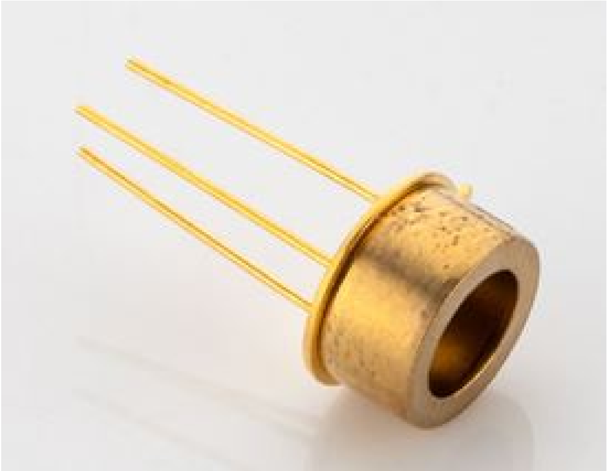
2 - 12um HgCdTe Photovoltaic Multi-Juncton IR Detector, PVM-10.6-1x1-TO39-NW-90
