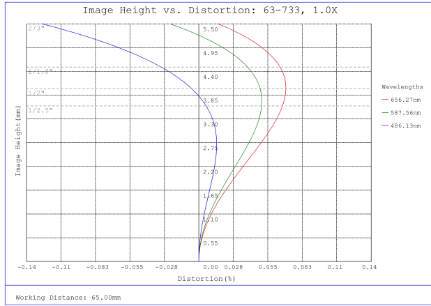
#63-733, 1X, 65mm WD CompactTL™ Telecentric Lens, Distortion Plot
