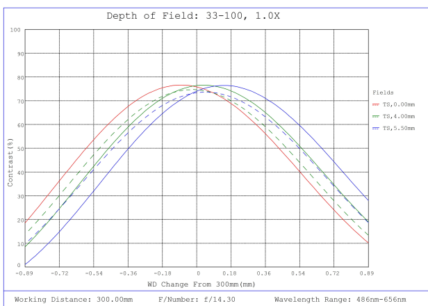
#33-100, 1X, 300mm WD CompactTL™ Telecentric Lens, Depth of Field Plot, 300mm Working Distance, f14.3
