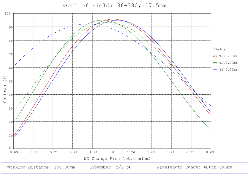
#36-380, 17.5mm FL f/2.5, Rugged Blue Series M12 Lens, Depth of Field Plot, 150mm Working Distance, f2.5
